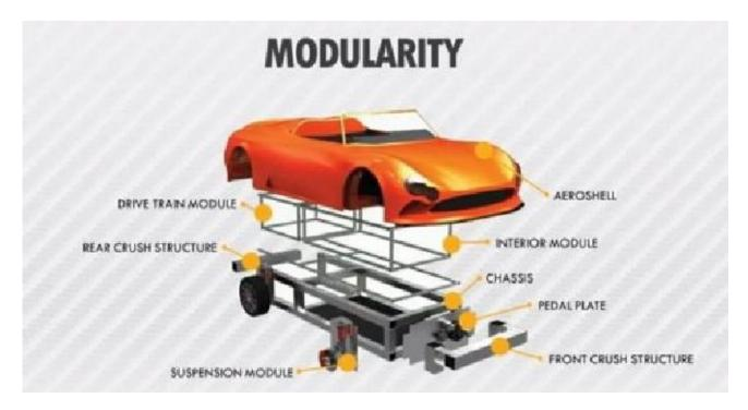
Fig. 4: The Wikispeed modular design (Source: Tincq 2012)
